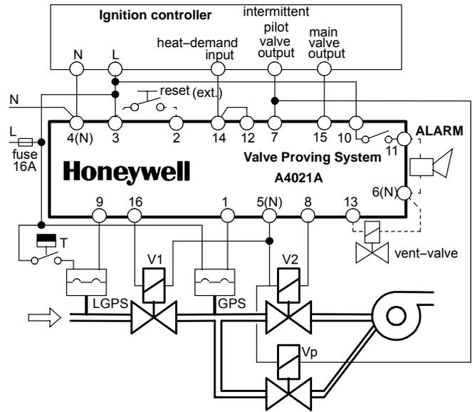
Fig. 12. wiring diagram 3-valve configuration (pre-configuration)
