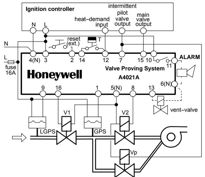
Fig. 13. Wiring diagram 3-valve configuration (post-configuration)
