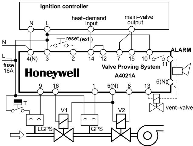
Fig. 10. Wiring diagram for 2-valve configuration pre-configuration
