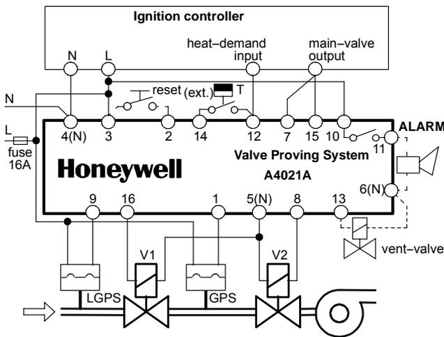
Fig. 11. Wiring diagram 2-valve configuration for post-configuration
